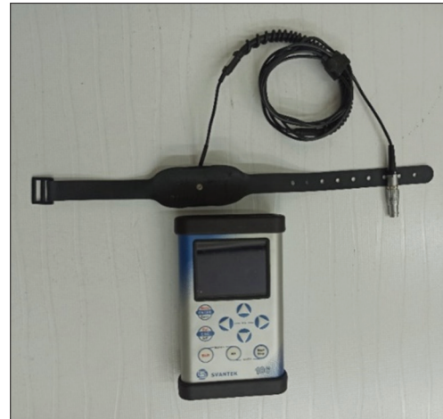
Figure 1: Hand-transmitted vibration measurement device used in the study
