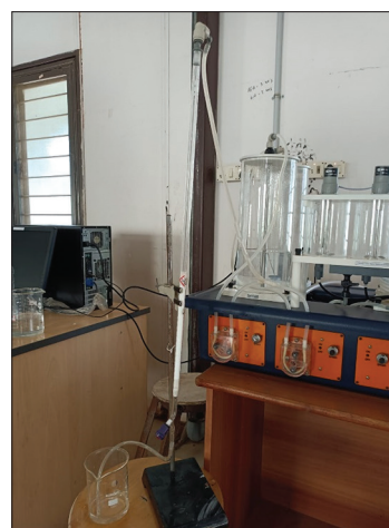
Figure 2: Photographic image of continuous column for adsorption of fluoride in aqueous solution in our laboratory
