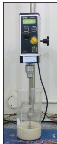
Figure 1: Drilling fluid preparation
