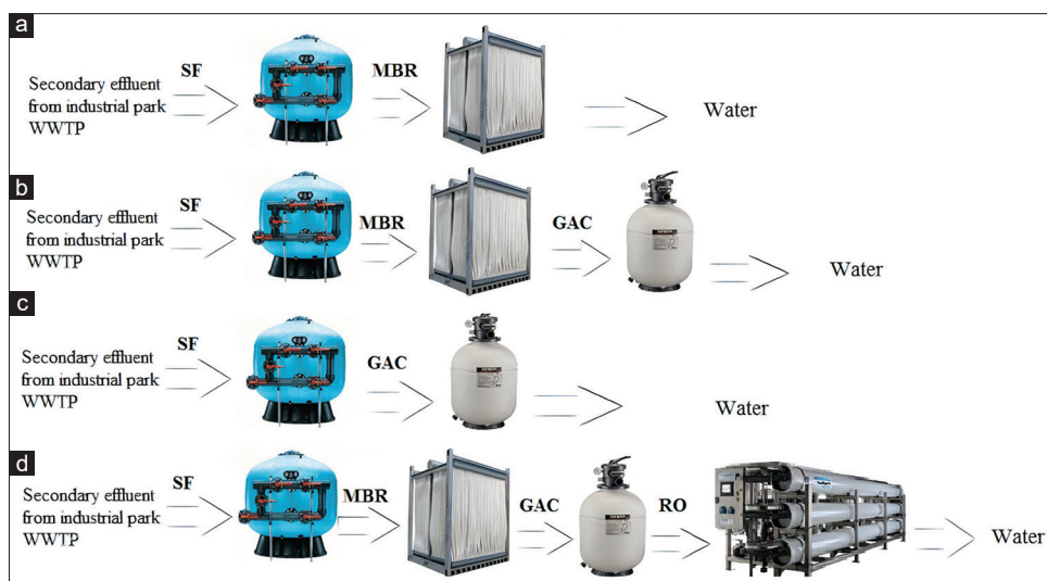
Figure 2: Scenarios of hybrid advanced system in the industrial park (a) scenario 1, (b) scenario 2, (c) scenario 3, (d) scenario 4
