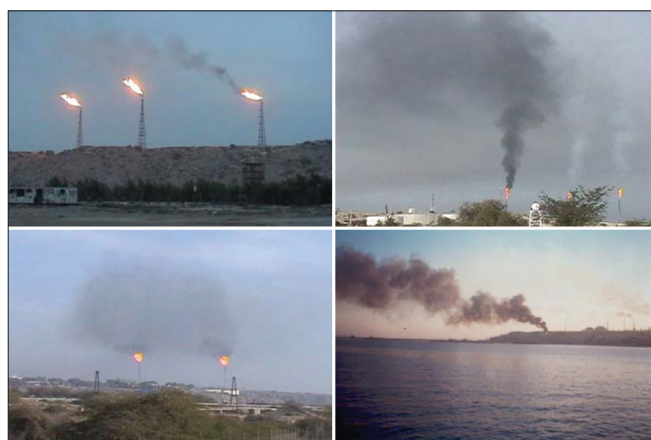
Figure 1: Burn extra fuels and smokes caused by imperfect gas combustion
