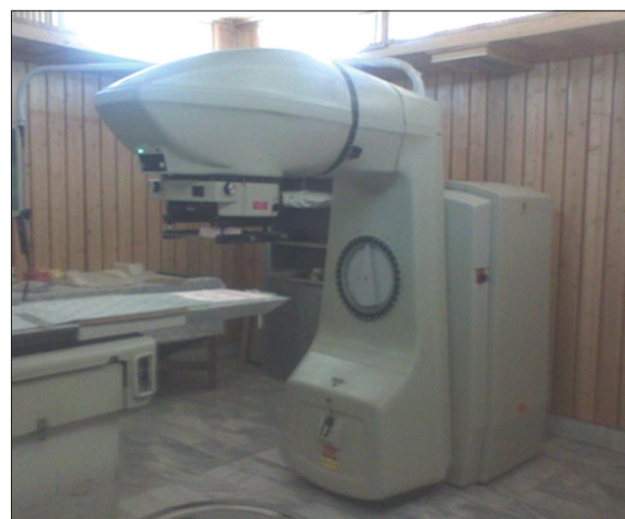
Figure 1: The 60 Co equipment used for irradiation of the samples
