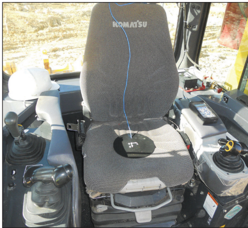
Figure 1: Placement of vibration accelerometer on equipment seat
