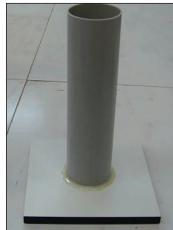
Figure 3: Designed PVC Helmholtz resonator
