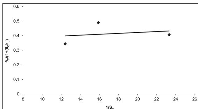
**Figure 3:** Determination of  $\mu_{max}$  and  $K_s$  coefficients in A-stage
