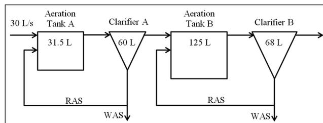
**Figure 1:** Schematic diagram of pilot-scale A-B process
