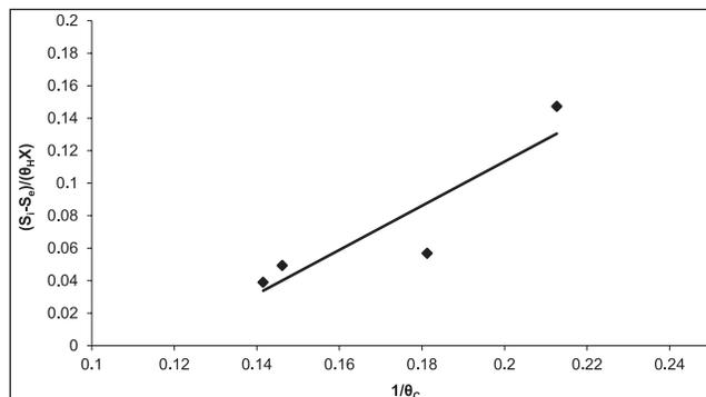
**Figure 4:** Determination of  $Y$  and  $K_d$  coefficients in B-stage
