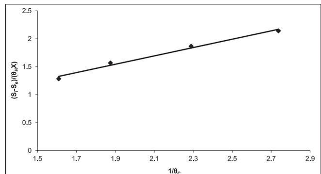
**Figure 2:** Determination of Y and  $K_d$  coefficients in A-stage
