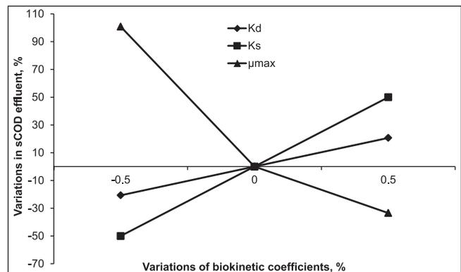
Figure 7: Sensitivity analysis of biokinetic coefficients of B-stage
