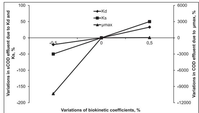
Figure 6: Sensitivity analysis of biokinetic coefficients of A-stage
