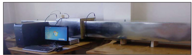
Figure 3: Laboratory Setup for determine sound pressure level and the location of the two microphones in channels
